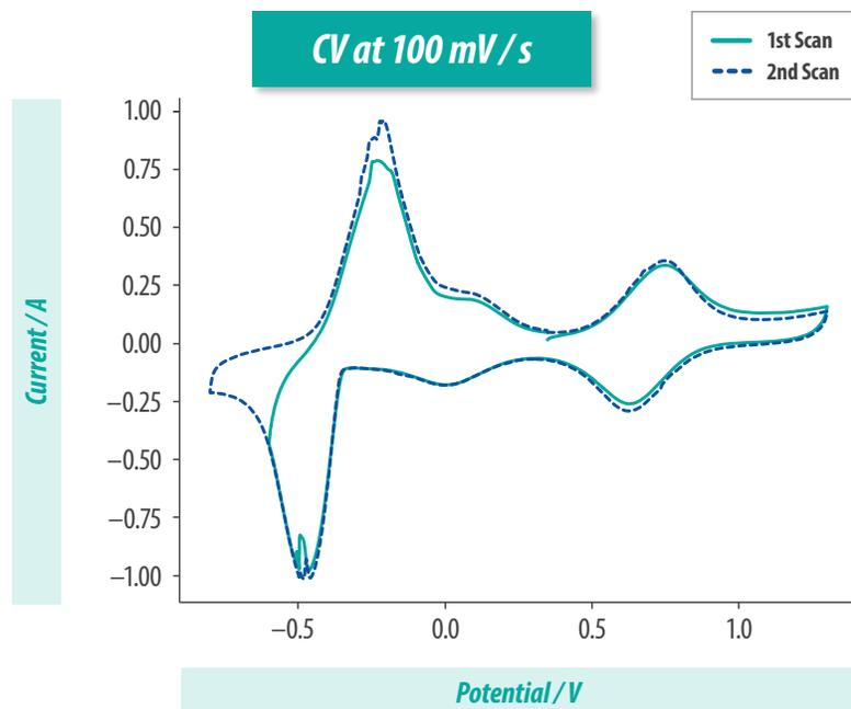
Cyclic voltammogram (CV) data demonstrating the bell-shaped curves returning to baseline current that is typical for electrochemical reactions with no mass transfer.
