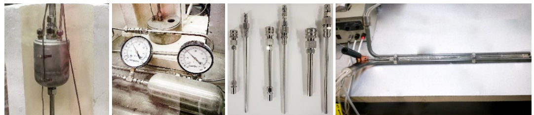
Figure 1 – Automated Molten Salt System for engineering scale electrorefiner: vacuum filled chamber (left), charge tanks (center left), charge tube assemblies with mating couplers (center right), sampling line with three-zone heater (right) From ref. 1.
