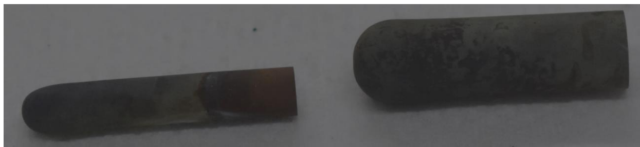
Figure 5. Pictures of two U- \beta'' alumina tubes (e.g., both with 1 mm wall thickness) made by ion exchange in \text{UCl}_3 salt at 735°C for 120 hours.
