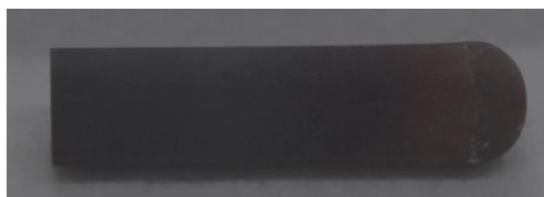
Figure 7. A picture of a Na-β'' alumina tube (e.g., 6.5 mm ID, 0.5 mm wall, and 30 mm long) that was ion-exchanged in salt vapor above UCl 3 salt. No water cleaning and annealing were used after the ion exchange.
