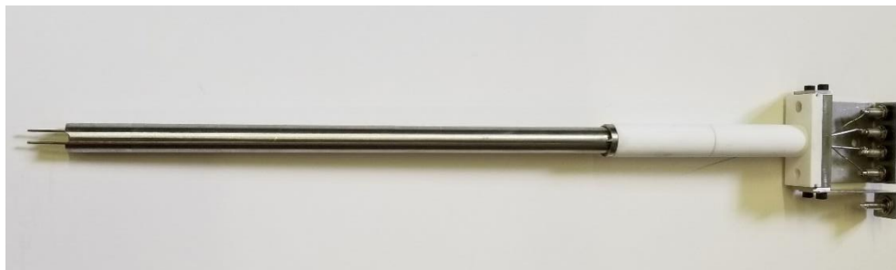
Figure 1. Photo of the OR voltammetry probe used in field-testing.
