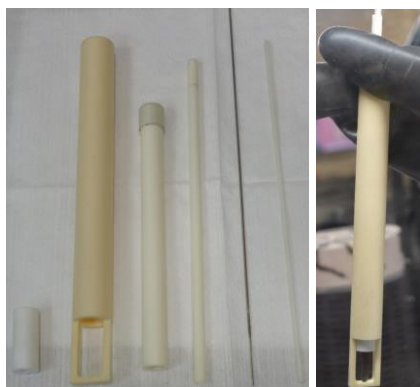
Figure 4. Picture of components for assembling a U-sensor electrode and a U-sensor electrode ready for testing.
