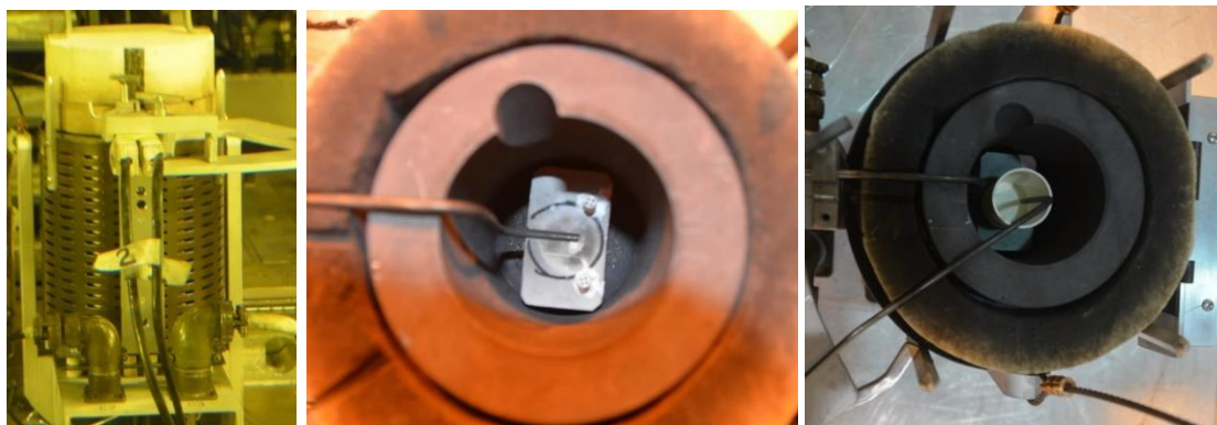
Figure 14. Pictures showing: (a) the furnace inside a hot cell in argon atmosphere; (b) the location of external thermocouple in grooved alumina block; and (c) the internal thermocouple inside of a yttria crucible.
